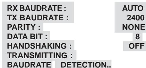
Figure 35: TRANSMIT [TX] TEST Display
